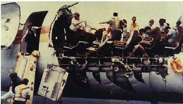
Aloha Airlines, Flight 243, April 28, 1988 became known around the world as “the convertible” when it lost 18 feet of the upper fuselage at 24,000 feet. Only one person out of the 95 on board lost her life but the world demanded to know how this could happen to a modern jet transport. This was not the first Boeing 737 to have this type of
