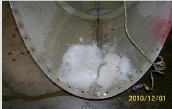
The mandatory actions prescribed in the letter advised operators to look for drain holes in frames immediately forward and aft of access panel 321ABC and to drill them if not present. The letter also instructed operators to drill a drain hole in the aft canted bulkhead. According to the NTSB's preliminary report, the Excel involved in the March 10, 2011 incident had been modified to comply with the ASL.
