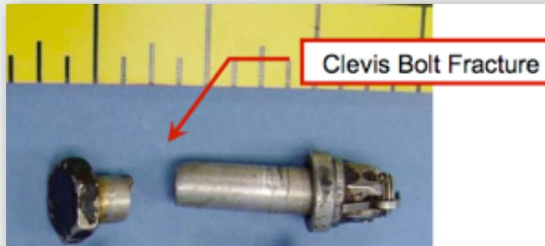
The bolt in question was one of two that anchor the complex mechanism that operates the helicopter's rotor blades, transmitting the pilot's flight commands to the blades that control the aircraft's direction.
