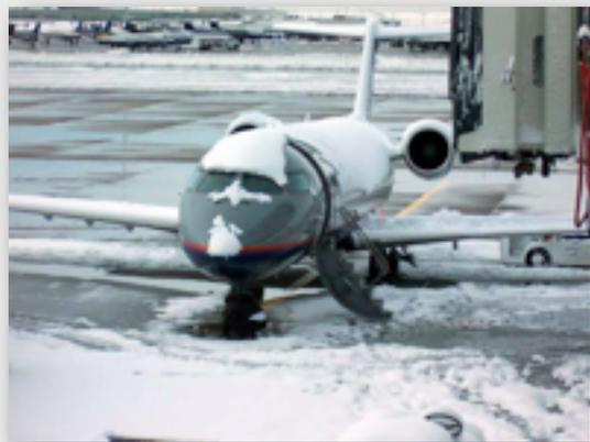
**Extreme caution** also is needed when towing an aircraft due to the added weight and the fact that most of the time you are relying solely on the braking action of the tug to stop both the aircraft and the tug. On wet, slick or icy surfaces the aircraft in tow can suddenly jack knife out of control as you turn or attempt to stop.
